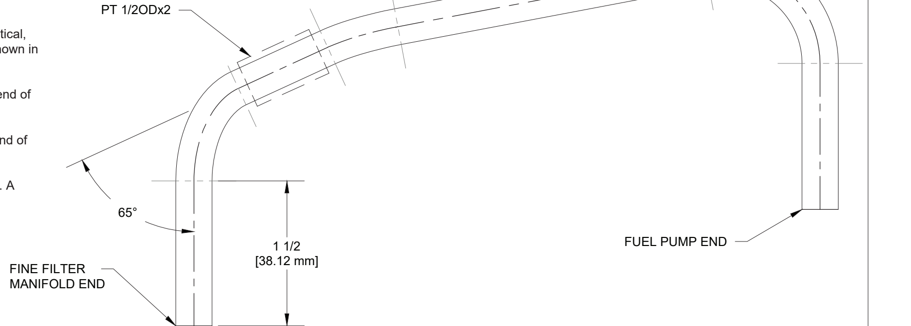
FIGURE 1: F-12127R PUMP TWO TO FUEL PRESSURE SENSOR THIRD BEND (NOTE: CHECK PRINTED SCALE 1:1 PER SECTION 3 BEFORE USING THE TEMPLATE!)
