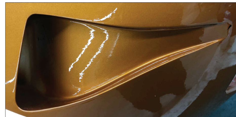
FIGURE 3: FINISHED ENGINE AIR INLET
