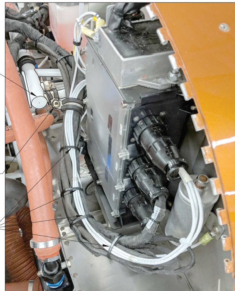
FIGURE 3: SECURING THE FUSEBOX WIRING
