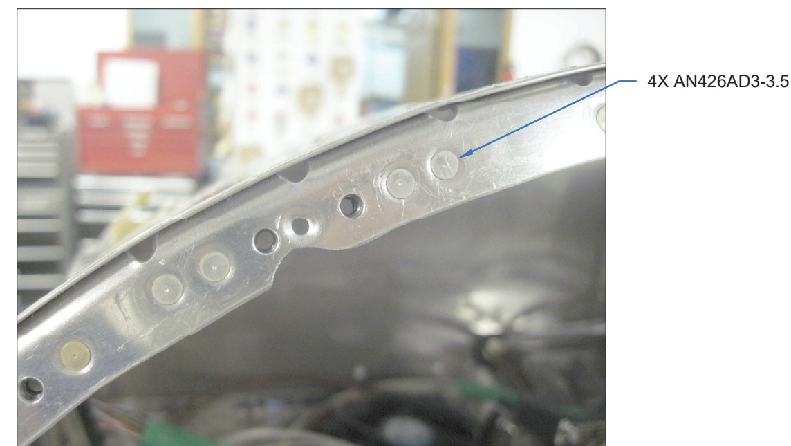
FIGURE 3: RIVETING THE NEW NUTPLATES
