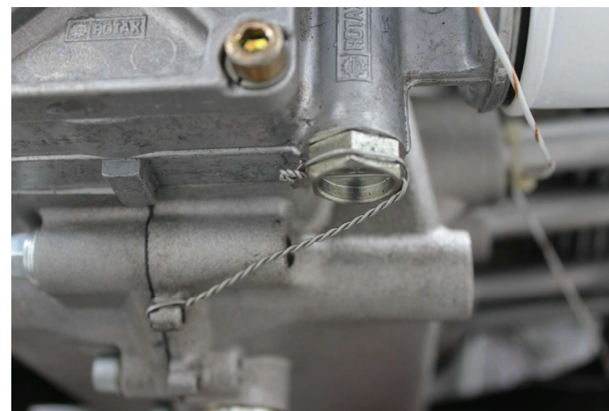
FIGURE 4: SAFETY WIRE OIL PRESSURE REGULATOR PLUG (912ULS SHOWN, SIMILAR FOR 912iS EXCEPT HOLE IN ENGINE PUMP HOUSING)
