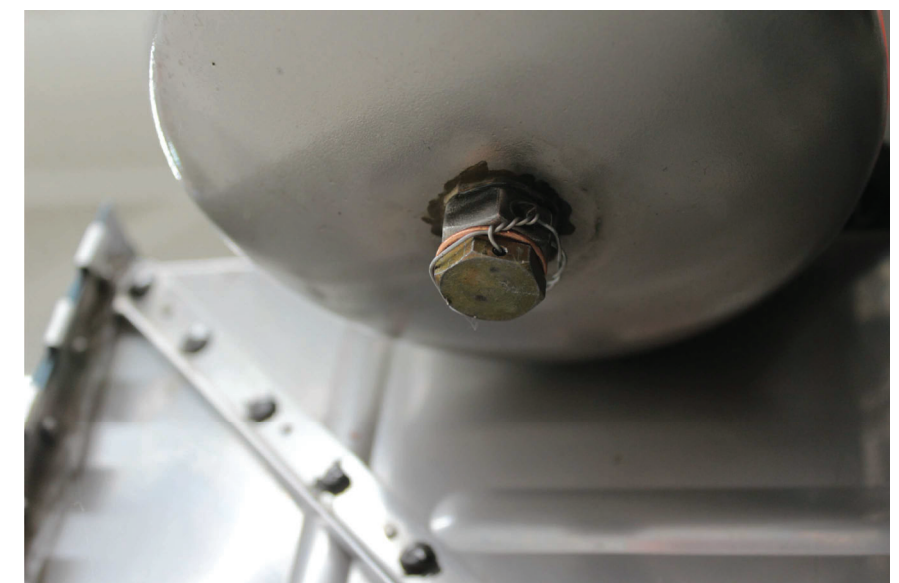
FIGURE 5: SAFETY WIRE OIL TANK DRAIN PLUG
