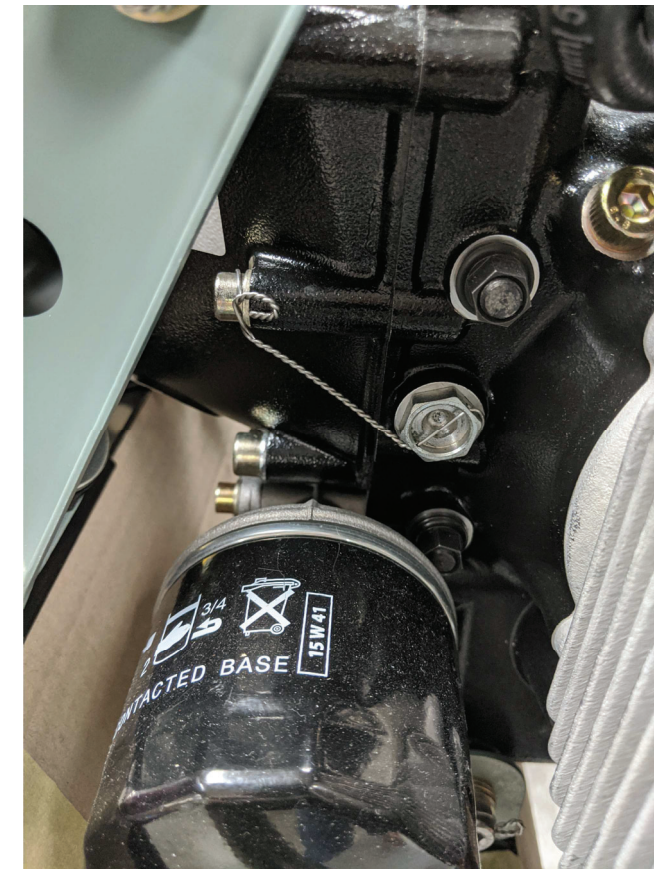
FIGURE 2: SAFETY WIRE MAGNETIC PLUG
