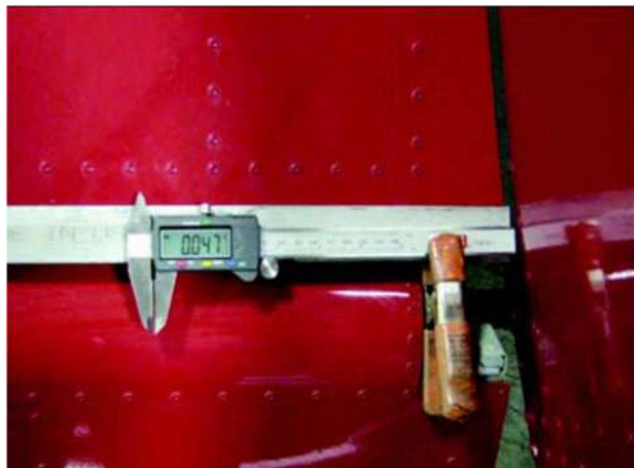
Figure 7.1: Inspect Rear Spar Doubler
